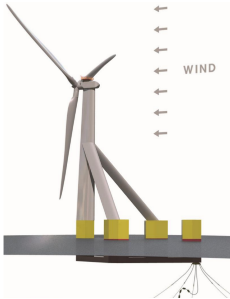
15 MW state-of-the-art wind turbine on floating platform Self-adjustment to wind direction
