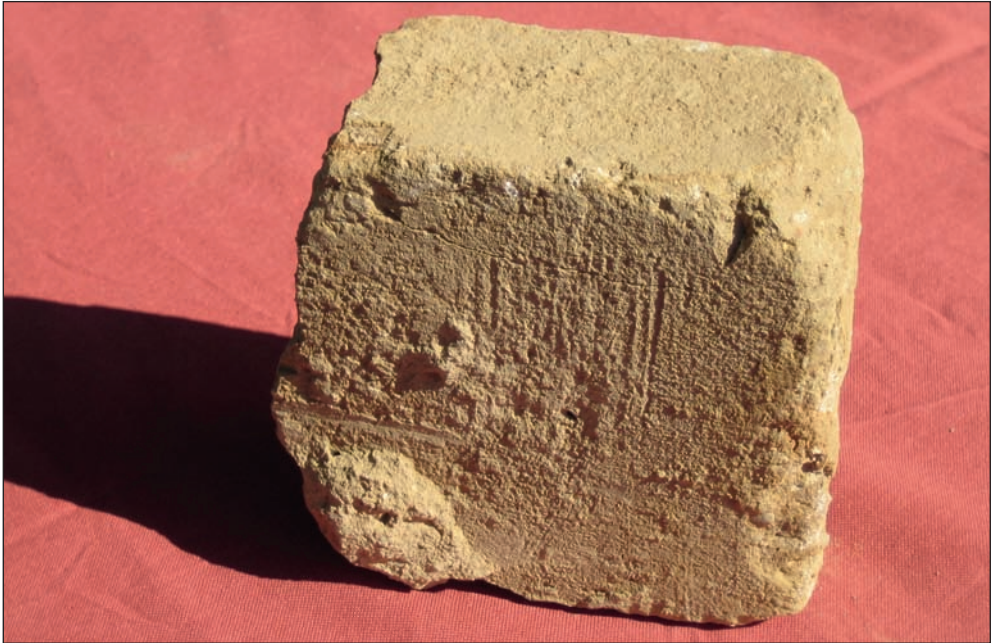
Fig. 12 Adobe of a wall inside a farm-worker house (Müncheberg, Brandenburg Province, Germany). Photo: C. DALCHOW
