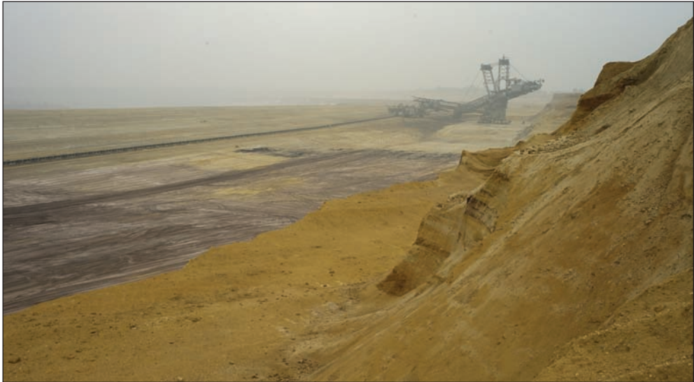
Fig. 5 Extraction and exchange of soils and rocks by humans: huge pits are opened first, coal is extracted then, and mixed rock and soil particles are filled in the pit. Finally fertile material is deposited on the top. The procedure is called “recultivation”, the soil type Anthrosol. (Vicinity of Jülich, Rhineland, Germany). Photo: H.-R. BORK
