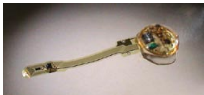
Fig. 2 The implant consists of an electrode array, which is connected to the control unit with a flexible foil conductor. The control unit is placed extraocularly sub-tenon (© IMI Intelligent Medical Implants GmbH).
