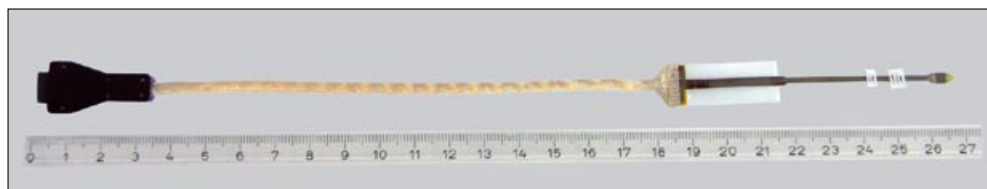
Fig. 1 Photograph of the active subretinal implant. It consists of four parts: (i) The subretinal part (polyimide foil strip, 20 \mu\text{m} thick, 3.2 mm wide, approximately 22 mm long) with: a 4 \times 4 array of titanium-nitride electrodes (diameter 50 \mu\text{m} , spacing 280 \mu\text{m} ) and a microphotodiode array with 1,550 photodiodes and electrodes (electrode diameter 70 \mu\text{m} , spacing 70 \mu\text{m} , thickness 70 \mu\text{m} ) which lies para-foveally. (ii) The extra-ocular part (polyimide foil) carrying 22 golden connection lanes to the external connection and the reference electrode. At length 12 and 26 mm from the tip two polytetrafluoroethylene pads are mounted for fixation on the sclera. At approximately 55 mm from the tip a silicone pad is glued to the polyimide foil for suture fixation to the lateral orbital rim. (iii) The subdermal part (silicone cable, diameter 3 mm) leads the connections on the polyimide foil to the external part by 22 spiraled gold flexes. The silicone cable perforates the retro-auricular skin. (iv) The external part consists of the silicone cable which connects via a plug to an external generator for control signals, energy, and stimuli.
